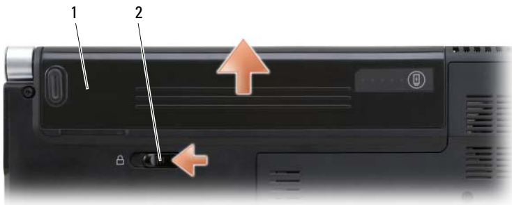
1 battery 2 battery release latch
